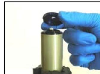
4. Remove the compression damper from the upper tube by pulling it up and rocking side to side. Once removed, clean the upper tube threads with a rag.
