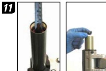
12. Clean the top cap, then apply a small amount of grease to the top cap threads and o-ring. Insert the top cap into the upper tube/crown and hand thread it into the upper tube. Be careful not to damage the top cap o-ring upon installation. Use a 24 mm socket wrench to tighten to 7.3 N-m (65 in-lb).
